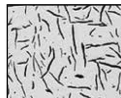
Graphite flakes in the microstructure of the XG-150 cast iron
